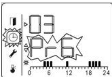
After confirming the end of the third COMFORT period, the system automatically exits the setup mode to the main user menu.
