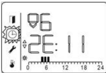
The program switches to the mode for selecting the hour of the end of the second period COMFORT.
